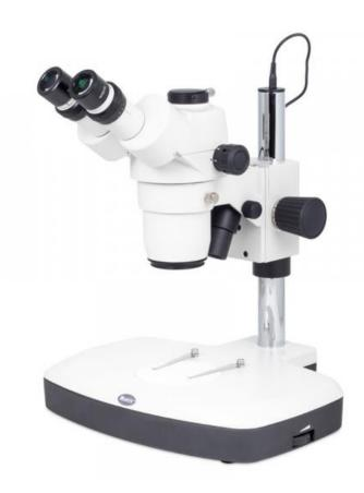
A versatile Trinocular stereo microscope for a wide range of biological and material science applications in both routine and research fields. The Greenough optical system delivers impressive images in a parfocal 6.7:1 zoom. The standard magnification range of 7.5X-50X is the basis of a durable workhorse. Students and lab technicians benefit from the package solution with integrated 3W Transmitted/Incident LED illumination.
