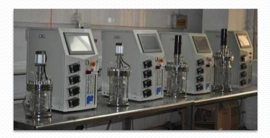
The fermenter plant offered is comprising fermenter designed and built for a broad range of modern fermentation applications.
